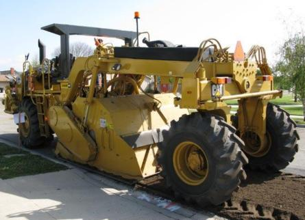
AC and underlying materials are pulverized and mixed to provide a homogenous base material. Additional aggregate may be incorporated to adjust gradation.
